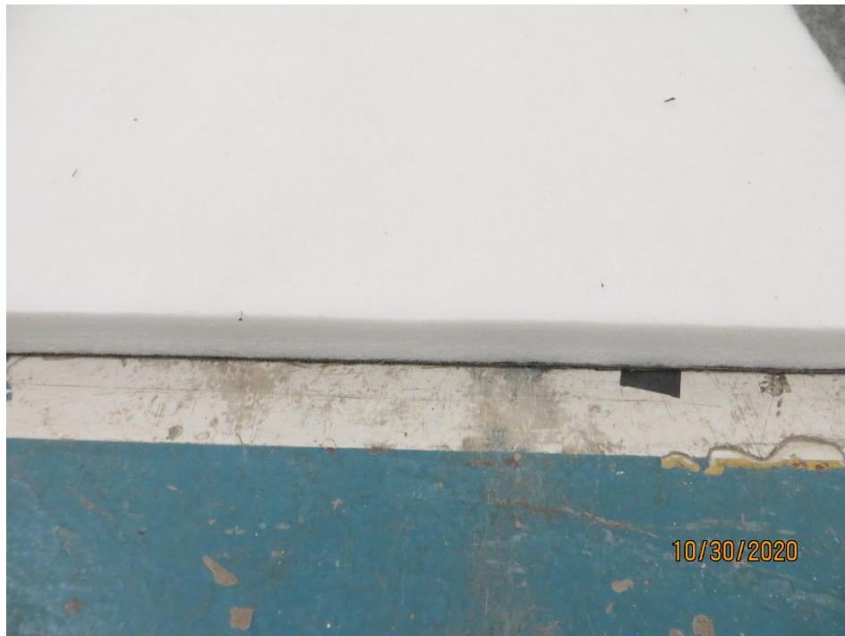
Figure 3 – Detail of specimen installation, mass loaded vinyl layer mated to test surface
